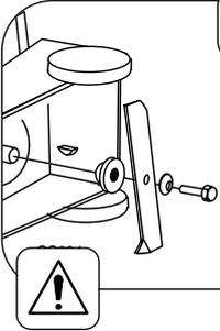
Assemble the cutterblade with the turned up edges facing towards the engine. Secure the cutterblade using the bolt, spring washer, and distance piece and tighten to a torque of 54Nm.
