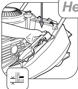
Hold the trigger against the handle and raise or lower the mower using the handle to achieve the desired height of cut. Release the trigger to secure the mower at the required position.
