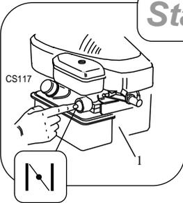
**Operate the primer bulb:** *Note: Push on the primer bulb 5 times at two second intervals to provide the extra fuel to start the engine after assembling the mower for the first time.*
