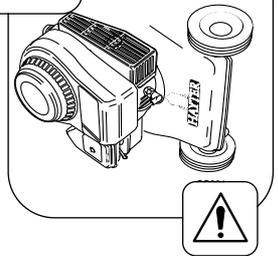
The condition of the cutterblade and its mounting arrangement should be checked regularly for signs of wear or damage. Ensure that the cutterblade is not bent or cracked.
