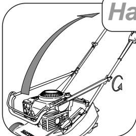
Unscrew the handlebar securing knobs sufficiently to allow the handlebar to pivot. Hold the engine stop lever in towards the handlebar and unfold the handlebar to the operating position, before releasing. Tighten both handlebar knobs to secure in position.
