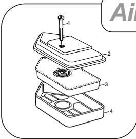
To service the air cleaner, remove screw (1) and remove cover (2). Carefully remove foam element (3) and wash in a solution of liquid detergent and water. Allow to air dry thoroughly before fitting or wrap in a cloth and squeeze dry. If very dirty, replace.
