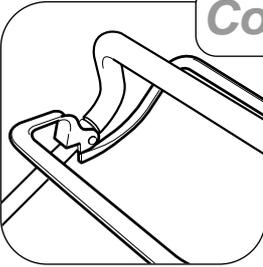
Operate all control levers several times and ensure that the cables move freely. Check that the engine stop and ground drive clutch levers return freely to their rest position when released.
