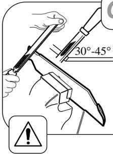
A slightly worn cutterblade may be re-sharpened. Both blade edges must be sharpened equally to ensure balance. Sharpen the cutterblade every 25 mowing hours or more frequently if conditions require. Remove the cutterblade from the mower and clean using a brush and water. Inspect the cutterblade for signs of damage. Sharpen both cutting edges with a flat file to restore performance.
